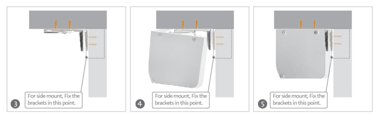
Step 3: Fix the mounting brackets with screws.
