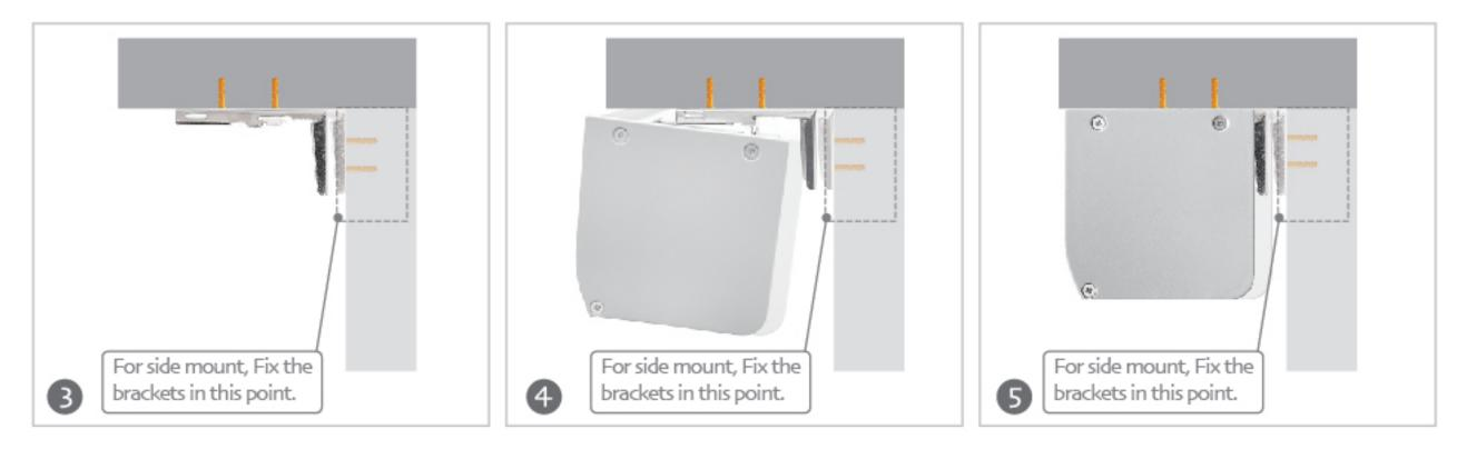
Step 3: Fix the mounting brackets with screws.
